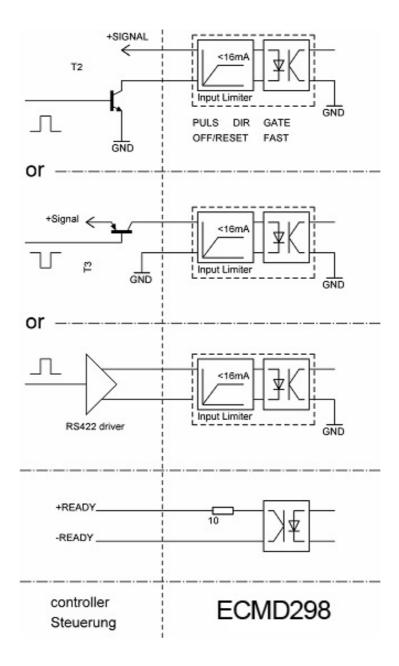
The signal interface is completely isolated by optoisolators. To have a wide flexibility, both inputs plus and minus of the opto-isolators are available. So its easy to drive the signal interface with high-, low- or RS422 active signals. All signals have a wide range voltage input and can be operated with signal voltage levels between  $3.5 \ensuremath{V}$  to  $24 \ensuremath{V}$
