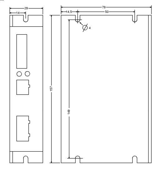
Dimensions: H:W:D: 157x29x79 D = 90 mm incl. Connector, W = 45 mm incl. Head Sink
