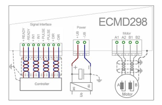
Motor connection bipolar parallel:
