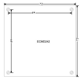
Overall height of the power drive including the PCB: 12mm
