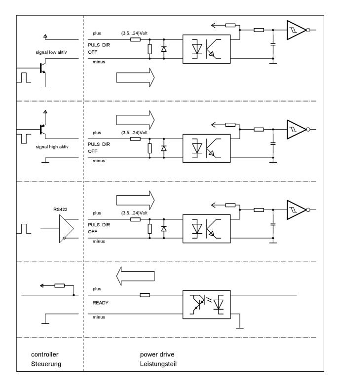
The signal interface is completely isolated by opto couplers. To have a wide flexibility, both inputs plus and minus of the opto couplers are available. So its easy to drive the signal interface with high-, low- or RS422 active signals.
